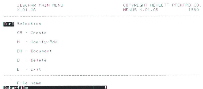
Fig. 5. A general principle of IDS/3000 menu design is that each word should convey important information.
